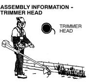
NOTE: Remove the blade before attaching the trimmer head. To remove blade, align hole in the dust cup with the hole in the side of the gearbox by rotating the blade. Insert a small screwdriver into aligned holes. This will keep the shaft from turning while loosening the blade nut. Remove blade nut by turning clockwise. Remove the screwdriver. Remove both washers and blade. See INSTALLATION OF THE METAL BLADE for illustrations. Be sure to store all parts and instructions for future use.
